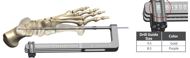
**Small Targeting Guide** (works with the 4.5mm Beams) – slide the Targeting Guide over the 2.0 mm Guidewire taking care to mate the beam with the external coupler. This coupler will engage the head of the beam and is locked into place by rotating the coupler in a clockwise fashion.
